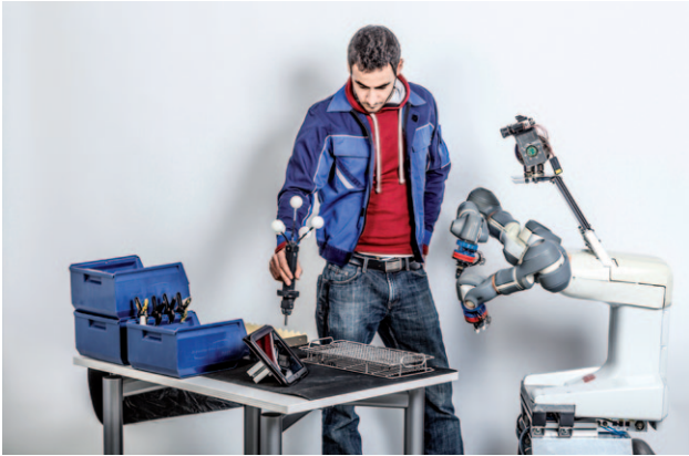
Figure 4: “Intelligent” dual-arm robot manipulation system to support the worker (Photo: Fraunhofer IPA/Rainer Bez)
