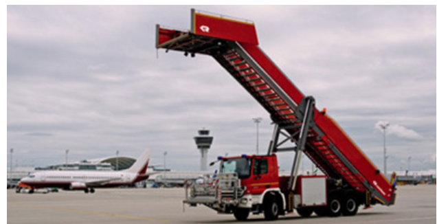
Figure 5: “Escape Stair” as a typical safety application (Photo: Rosenbauer)
