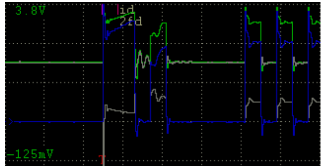
Figure 4: ID8 bit waveform with longer daisy-chaining cables
