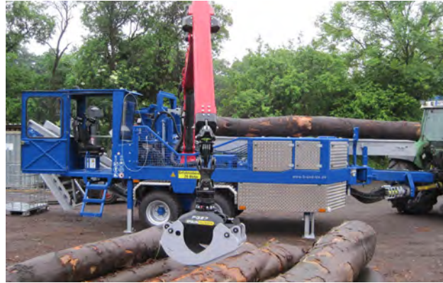
Figure 4: The tree trunk is sawed and split into handy logs; the control system calculates the lengths of the logs in such a way that all pieces have the same length and no unusable surplus remains left over
