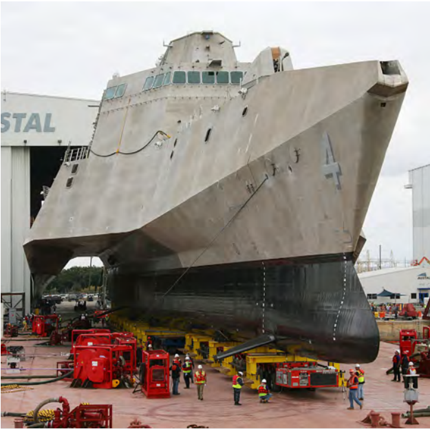
Figure 2: Safe and reliable transportation on land; the USS Coronado on Goldhofer PST/ES-E and PST/SL-E heavy-duty modules
