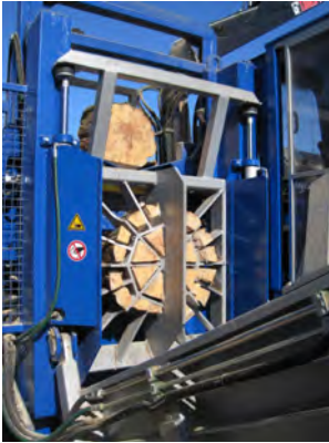
Figure 4: The tree trunk is sawed and split into handy logs; the control system calculates the lengths of the logs in such a way that all pieces have the same length and no unusable surplus remains left over
