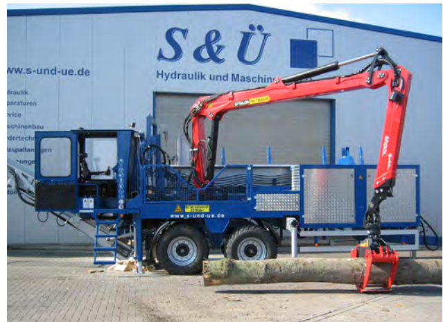
Figure 2: A crane is picking up the trunks, bringing them in the right position
