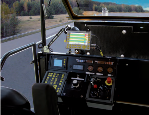
Figure 5: In cab display shows the progress of the paving
