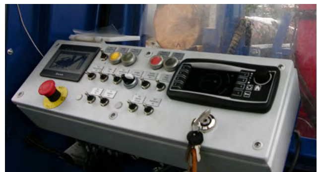
Figure 3: The panel on the right, an operating unit of the Opus series, controls the diesel drive and with the panel on the left, a control panel of the WBG series, the saw and split machine is controlled
