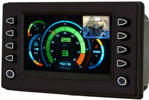
Figure 4: HMIs may convert the SI-Units to national units for convenience, but the CANopen devices must not communicate non SI-Units
