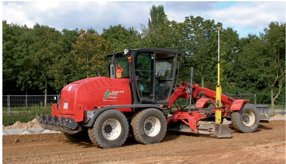
Figure 1: Grader working on a sports court in Southern Germany using the 3D-matic leveling system
