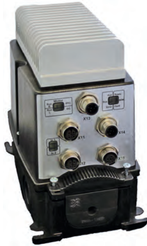
Figure 3: The Mono-Switch Fieldpower drive based on the Fieldpower box; the device has its own internal control logic and can therefore be operated without an overriding control system; the sensors are connected directly to the motor starter
