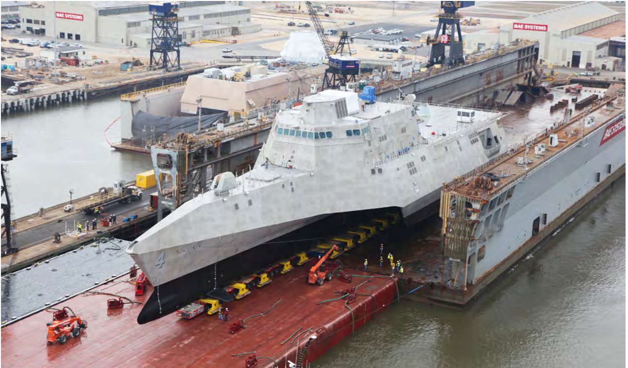
Figure 1: 2800 tons under one-man control; the complete 104-axle vehicle combination was steered by a single operator using a remote control
