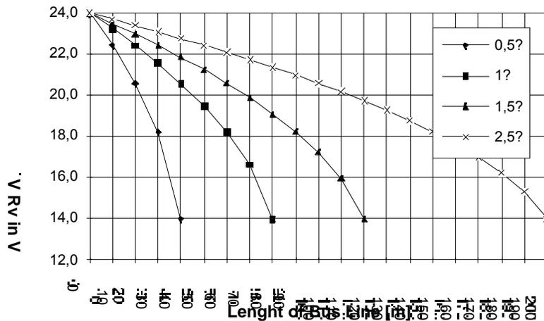
$$V_{R_v} = \frac{V_s}{2} + \sqrt{\frac{V_s^2}{4} - 2zR_L P_{BT}}$$
