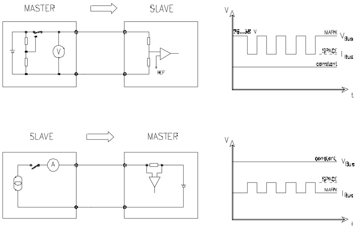
Figure 9: System structure of the Meter-Bus
