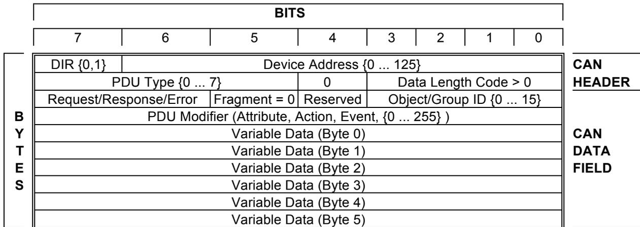
Figure 3 SDS™ APDU (long form) in a CAN Frame
