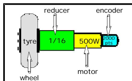
figure 3 :the encoder-motor-reducer set.
