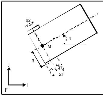
figure 4 : coordinates of mobile robot.
