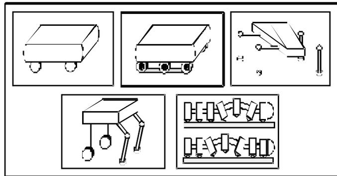
figure 2 : different locomotion structures in mobile robotics.
