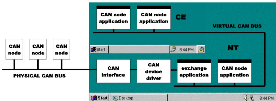
The virtual CAN bus environment does not provide true system timing accuracy, since all virtual CAN nodes run as multi-tasking applications on the same processor. For the same reason access to the virtual CAN bus does not support arbitration, but is handled purely on a first-come first-serve basis. Also no disturbances on the virtual CAN bus are provided now, but these can be very easily added.
