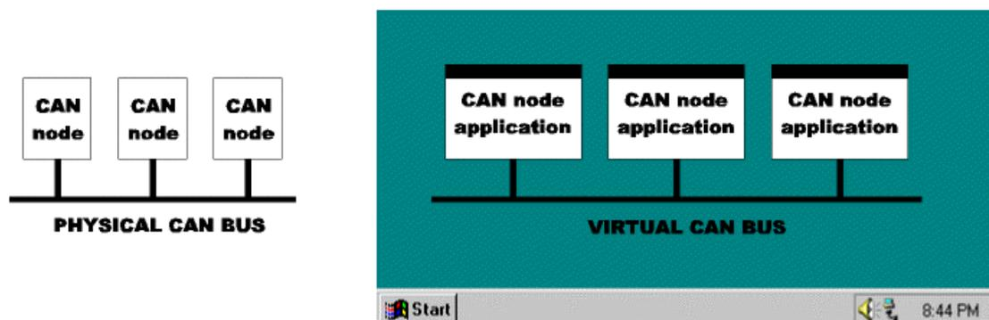
Because of the strict layering in the software of the CDE, it was rather easy to port the software modules normally taking care of message exchange via a physical CAN controller, to a mechanism in which the messages are distributed completely in software to other Window applications connected to the virtual bus.
