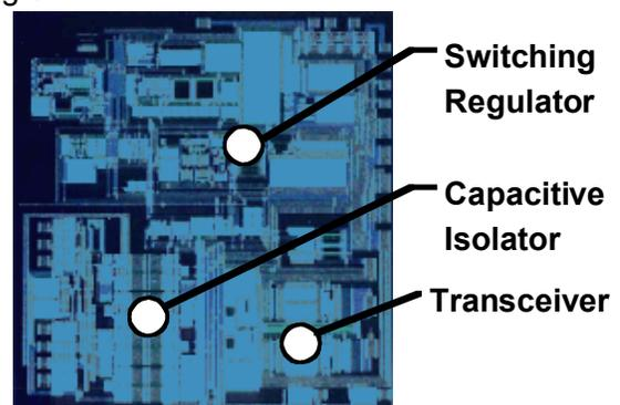
Fig. 7. Chip Micrograph.
