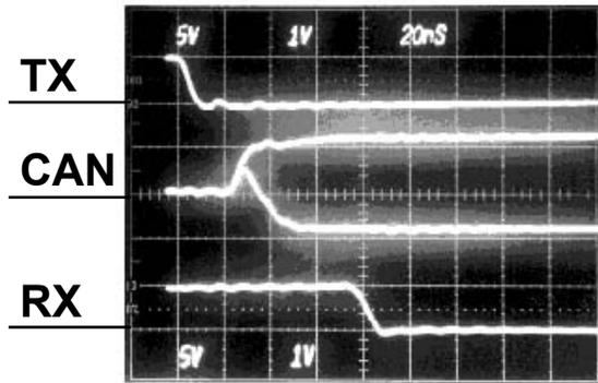
Fig. 8. TX to RX Loopback Waveform (Dominant).
