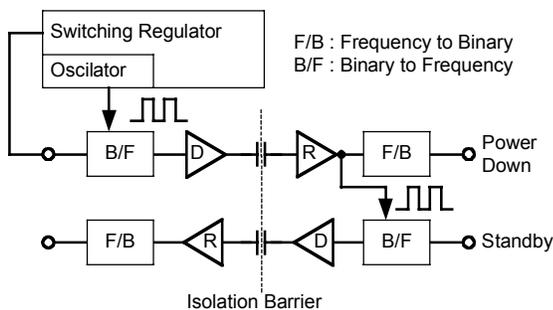
Fig. 5. Power Supply Monitor.
