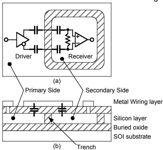
Fig. 4. Capacitive Isolator.
