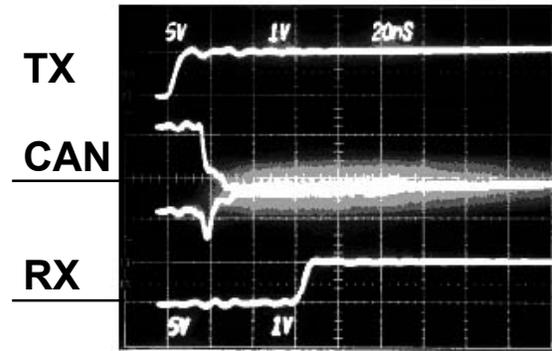
9. TX to RX Loopback Waveform (Recessive).
