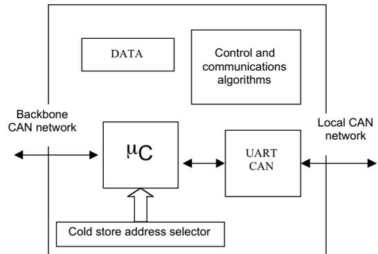
Figure 5. Central cold store nodes structure
