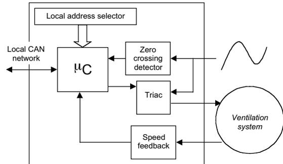
Figure 8. Ventilation control nodes structure
