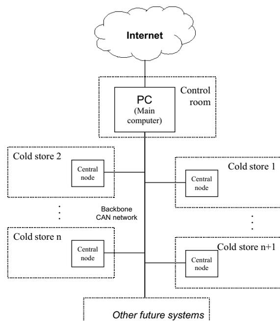
Figure 3. Hierarchy of networks and system architecture
