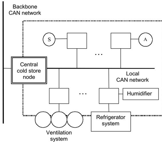
Figure 4. Central node and satellite nodes of a cold store
