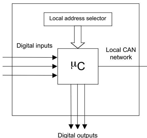
Figure 7. Digital I/O nodes structure
