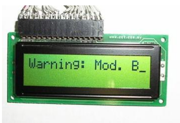
Fig.10 System Status Message - Module B does not work correctly
