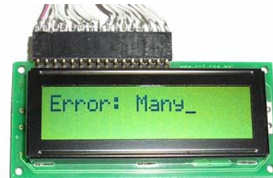
Fig.12 System Status Message – Module B and Module C do not work correctly
