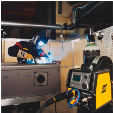
Figure 8: Welding equipment with a CAN-based, distributed control-system.
