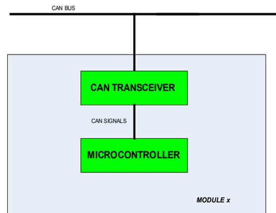
**Figure 5: Non-repeater modules have a single CAN transceiver and messages are interpreted on the microcontroller.**
