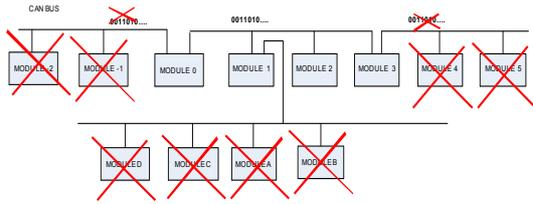
**Figure 9: Repeater example for multiple sub-busses**
