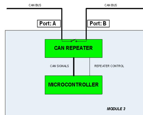
**Figure 6: The module with CAN repeater.**
