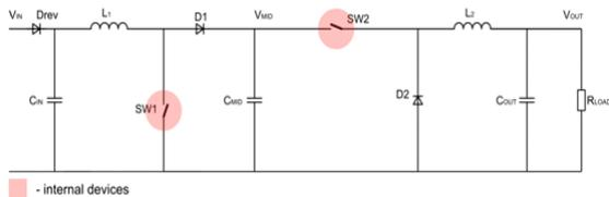
Figure 2: Principle drawing of Boost-Buck configuration in power SBC.
