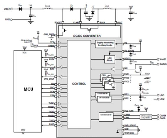
Figure 3: Example of an SBC based application using on chip LDO's and DC/DC converter.
