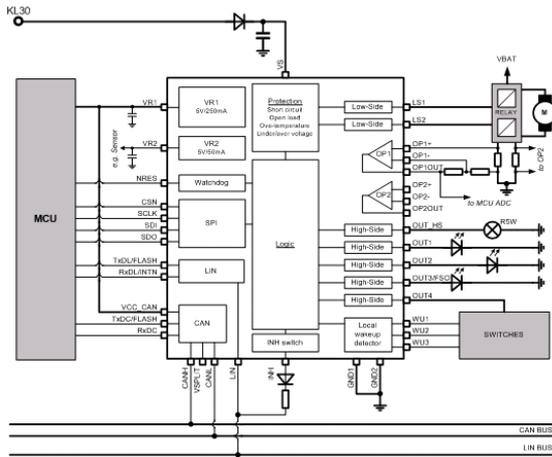
Figure 1: Example of an SBC based application using two on chip LDO's.
