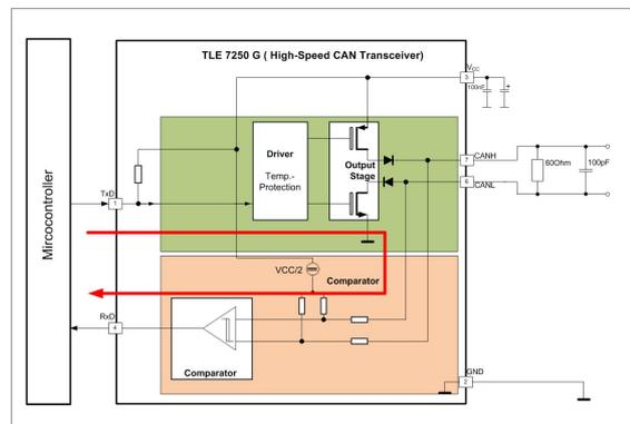
Figure 1: TxD to RxD Transceiver Propagation delay specification
