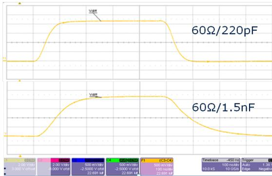
Figure 5: The impact of different capacitive load on the dominant bit time
