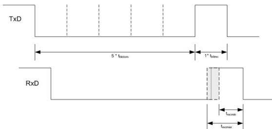
Figure 4: propagation delay specification for CAN FD transceiver
