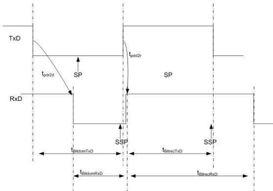
Figure 3: Transceiver with a very asymmetric propagation delay TxD to RxD
