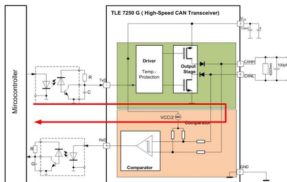
Figure 9: Optocoupler as interface for isolation
