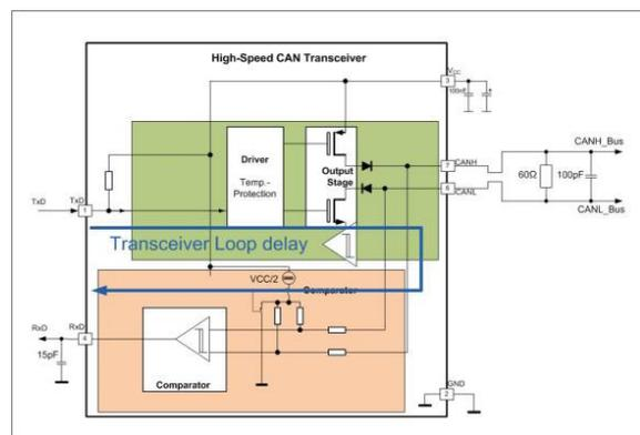
Figure 1: Transceiver Loop delay symmetry test circuitry
