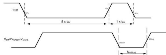
Figure 5: Transceiver Tx delay symmetry
