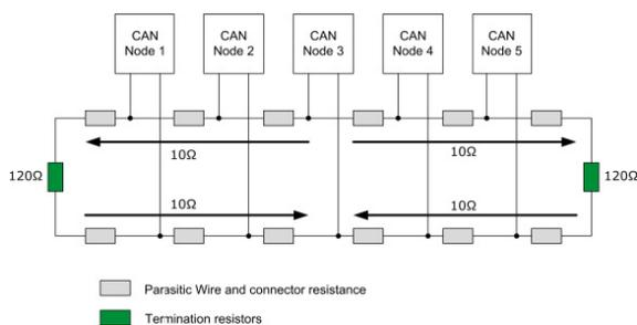
Figure 8: bus load for node 3
