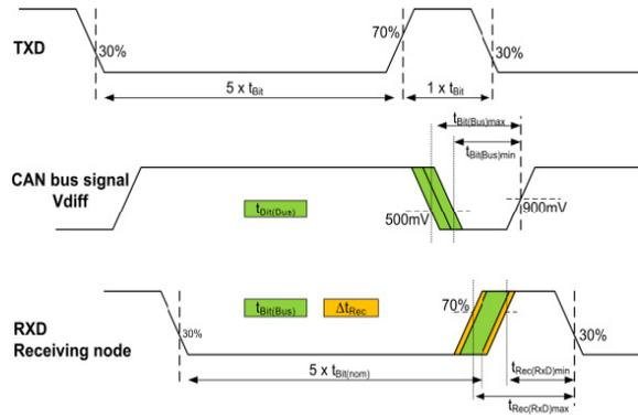
Figure 7: Recessive bit variation on a receiving node
