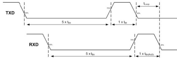
Figure 3: Transceiver loop delay symmetry specification
