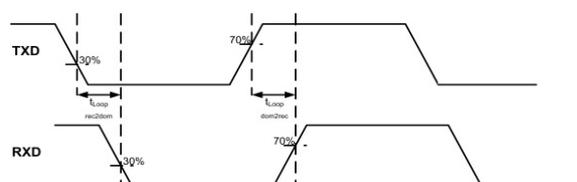
Figure 2: Transceiver Loop delay specification
