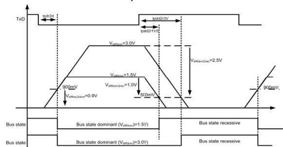
Figure 6: Dependency of Vdiff dominant voltage level and propagation delay symmetry
