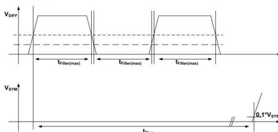
Figure 10: Bus bias reaction time definition
