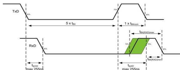
Figure 4: Transceiver Tx delay symmetry
