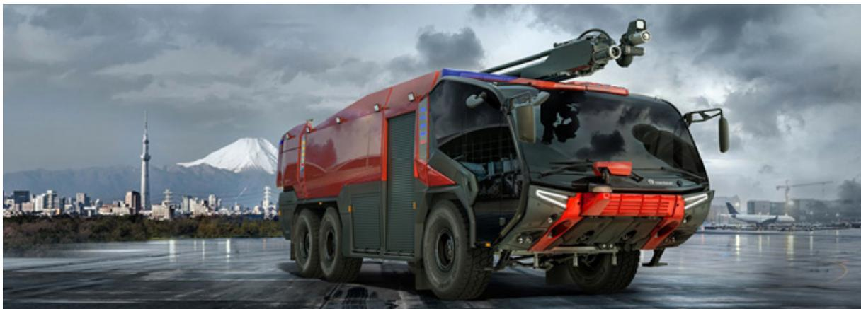
*Figure 1: 3-axle ARFF vehicle with boom (HRET)*
