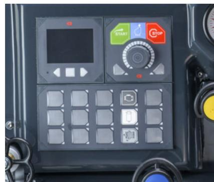
Figure 7: Operation via CAN key pane
