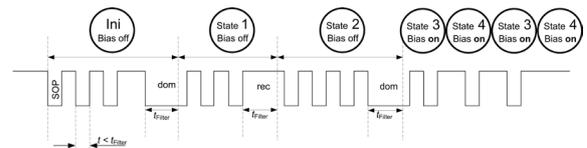
Figure 4: Wake up mechanism in a CAN frame
