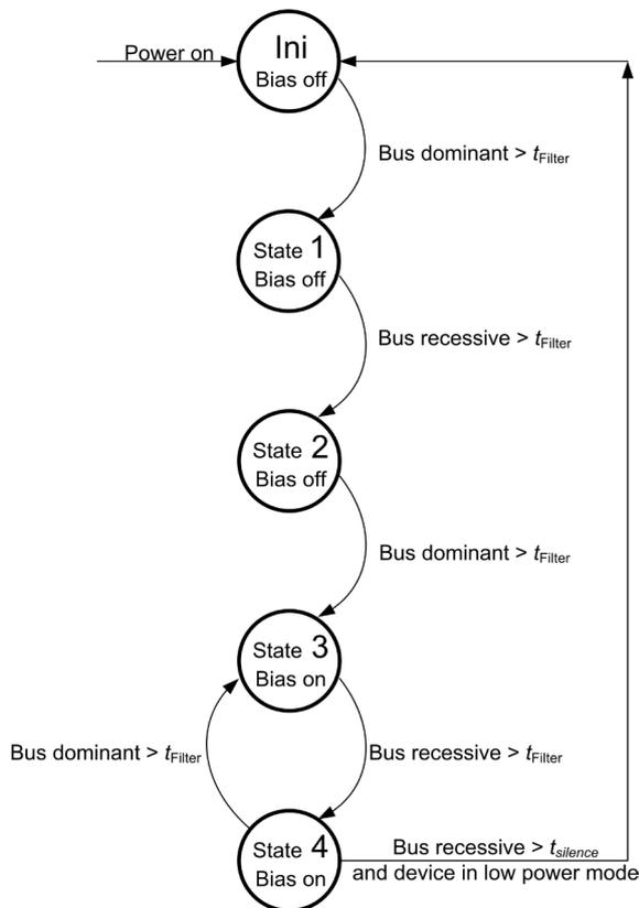
Figure 9: Permanent recessive level in State 4
