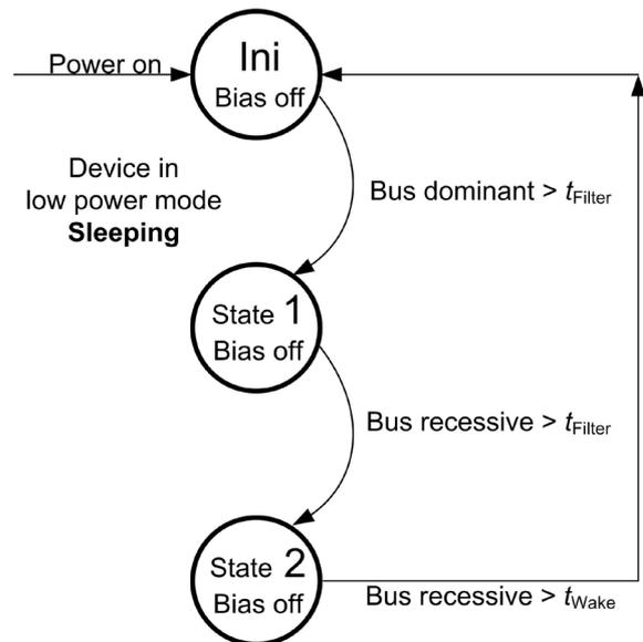
Figure 7: Permanent recessive level after a dominant spike
