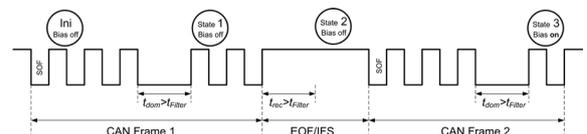
Figure 5: Wake up caused by two CAN frames
