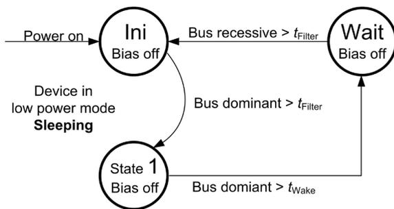
Figure 6: Flow for permanently dominant bus signal
