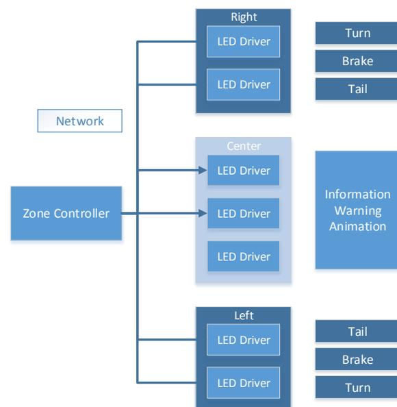
Figure 1 Rear Light Structure
